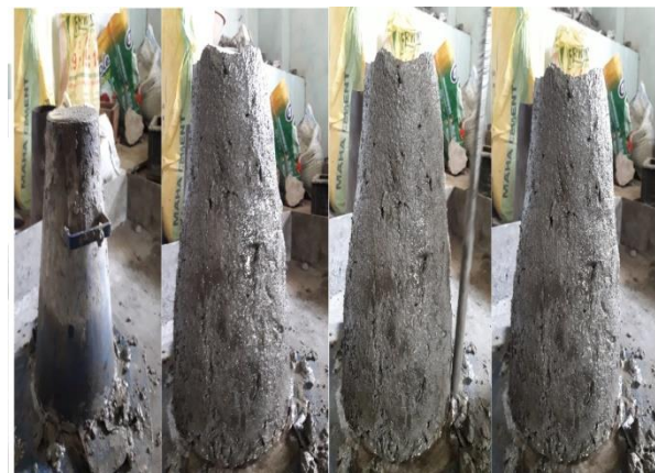
Figure 3: Slump Pattern of Concrete
